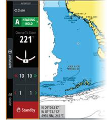
➔ **Note:** You switch the autopilot to Standby mode from any automatic mode by a short press on the WheelKey configured for Autopilot control.
