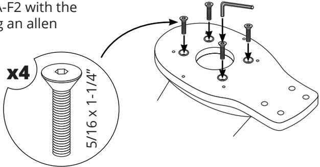
**4** Mount the FLIR M100 or M200 to the top of the adapter provided by FLIR.
