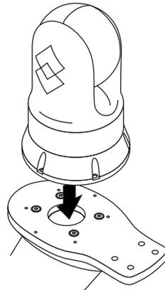
**7** Secure the adapter to the ADA-F2 top plate using the provided six #12 x 1" screws with a philips head screwdriver.
