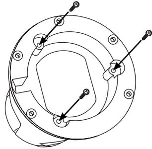
**6** Place the FLIR camera on top of the ADA-F2 top plate. Make sure that the six holes on the adapter line up with the six holes on the top plate.
