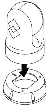
**5** Secure the FLIR M100 or M200 to the adapter with the hardware specified by your electronics manufacturer.
