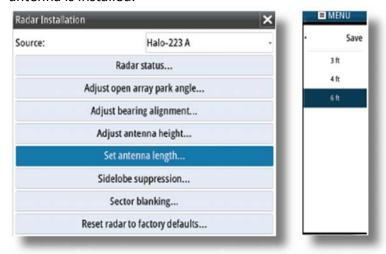
**Reset radar to factory defaults:** Resetting the radar to factory defaults is strongly recommended after the upgrade. This will not affect the installation settings such as antenna height and width. It will reset settings such as Gain and Sea Clutter.
