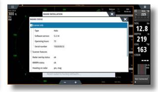
**Check antenna height:** Antenna height setting should be re-checked and confirmed as this is critical for STC/Sea Clutter optimisation.
