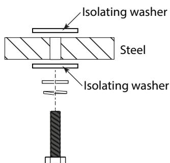
The eight hex head bolts supplied are suitable for surfaces up to 25 mm (1") in thickness.
