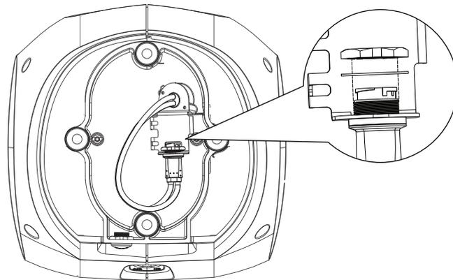
4. Connect the interconnection cable. Take care to align the connector correctly to avoid bending the pins. Secure the locking collar by rotating clockwise until it clicks.
