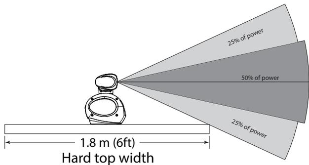
Below is a guide to determine the antenna height in relation to a vessels hard top overall width. Every Increase of 200 mm (7.9") of hard top total width over 1.8m wide: Increase the height of the antenna by 46 mm (1.8")
