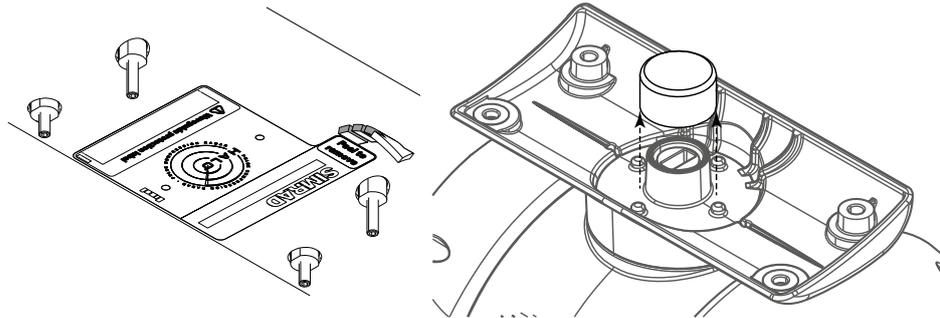
2. Carefully lower the antenna on to the pedestal. The antenna can only fit one way
