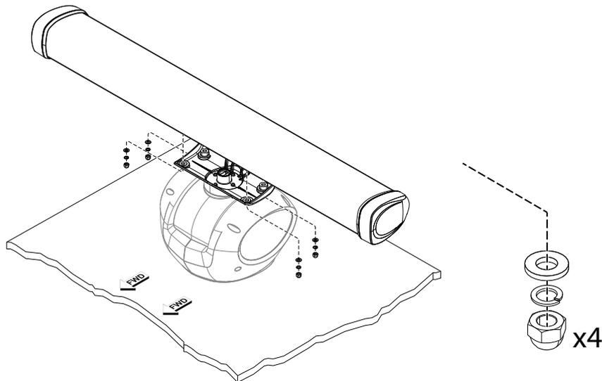
3. Place a flat washer then a split washer followed by a dome nut on to each of the four antenna studs. Tighten the dome nuts using socket and torque wrench to 15 N.m (11 ft.lbf)
