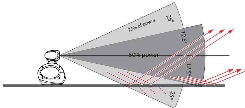
For best performance, the radar should be positioned to allow the beams to clear the superstructure of the boat.
