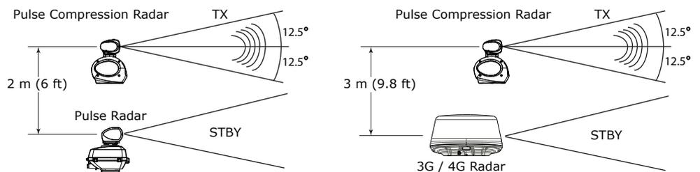
**Do not** install the Halo® pulse compression radar on the same beam plane as a conventional pulse radar. A pulse radar must be set to STBY or OFF any time the Halo® radar is being operated.
