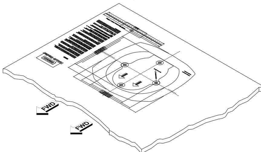
3. Drill pilot holes, Then use a 12.5 mm (1/2") drill bit to drill the four holes where shown on the mounting template.
