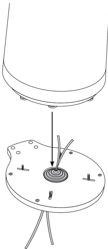
**6** Attach the lower adapter plate to the Seaview mount with the eight 5/16-18 x 1" bolts and nylon washers.
