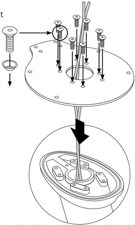
**7** Apply marine adhesive sealant to the circular groove on the under side of the adapter plate. Then place the adapter plate onto the lower adapter plate. Make sure that the bolt holes line up.
