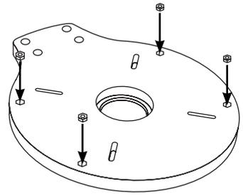
**2** Apply marine adhesive sealant along the lip in the center hole on the adapter plate.
