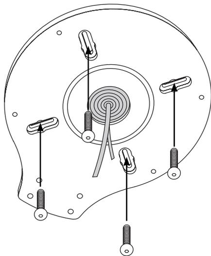
**5** Attach the satellite dome to the adapter plate, and secure with the hardware for your electronics.
