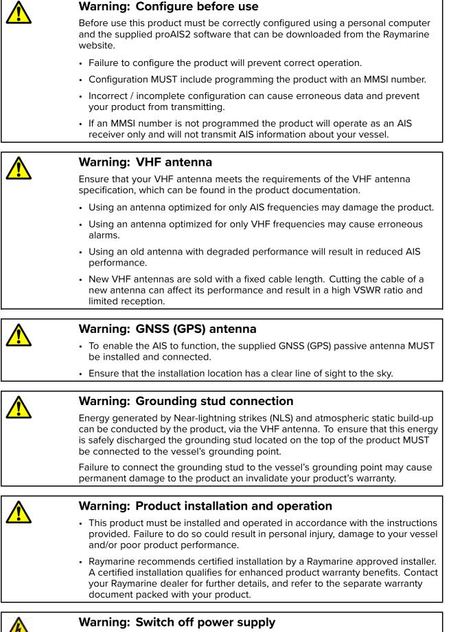
Ensure the vessel's power supply is switched OFF before starting to install this product. Do NOT connect or disconnect equipment with the power switched on, unless instructed in this document.
