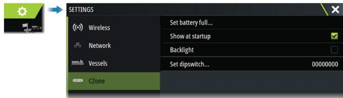
In order to communicate with the CZone modules connected to the network, the unit must be assigned a unique CZone Display Dipswitch setting.
