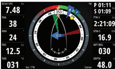
SailSteer provides a composite view of key sailing data. All data is displayed relative to the yacht's bow. The number of data fields included in the panel is dependant on available panel size.
