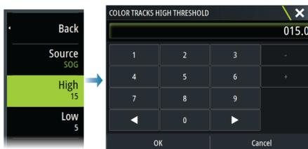
The colors can be shades of green, yellow, and red. Green is for the high limit you set. Yellow is the value that is the average of the high and low. Red is for the low limit. If the value is between the high and the middle values, it appears as a greenish-yellow color. If the value is between the middle and the low, it appears as an orange color.
