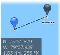
vessel moves, while the blue icon remains at the position given when you activated the function. The measuring points can then be repositioned by dragging either icon. Terminate the measuring function by selecting the finish measuring option.
