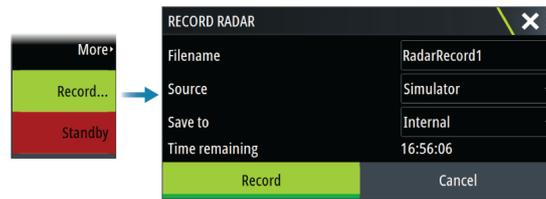
You can record radar data and save the file internally in the unit, or save it onto a storage device connected to the unit.
