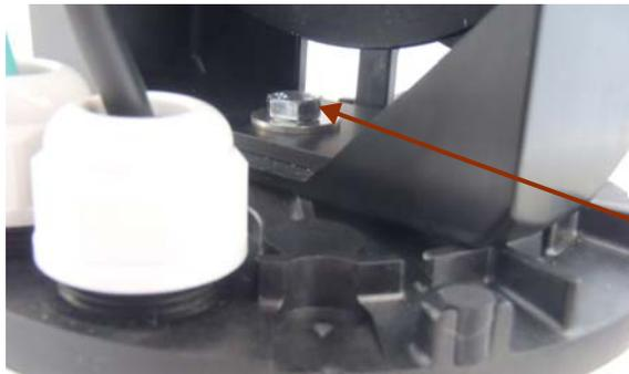
Loosen this bolt to remove camera from base
