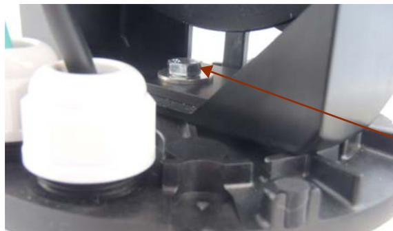
Loosen this bolt to adjust camera pan
