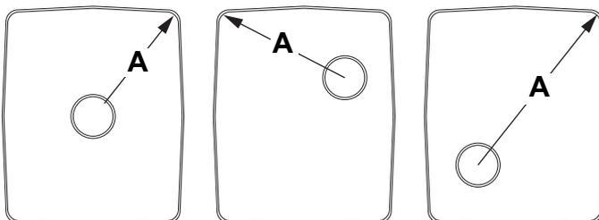
For every increase of 200 mm (7.9") of hard top distance over 1.8 m (6.0"), increase the height of the antenna by 46 mm (1.8").
