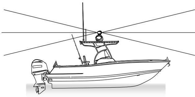
If you install your HALO radar on a power boat with a steep planing angle, it is recommended you tilt the radar angle down at the front.
