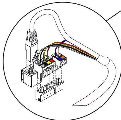
If you ever need to replace or refit the 8-pin RJ45 connector on the interconnection cable, use a RJ45 crimping tool and wire as follows:
