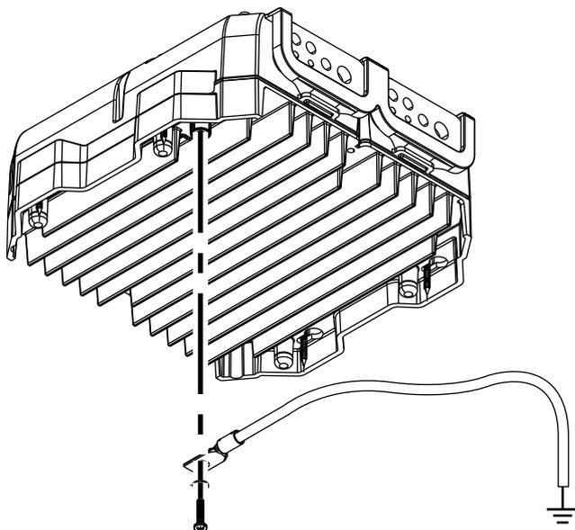
Alternatively, you can ground the RI-50 using the **CASE / SHIP GND** spade terminal on the circuit board.
