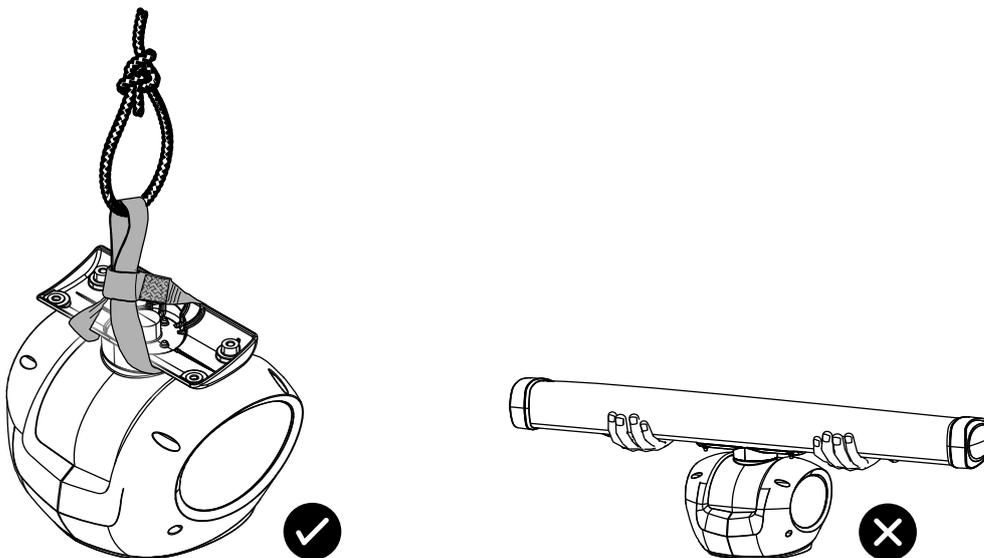
**⚠ Warning: Do not lift the pedestal with the antenna attached.**
