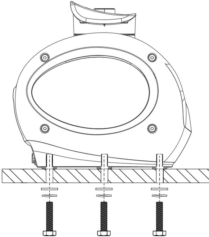
If you are installing the pedestal onto a steel surface, also use the supplied plastic isolating washers.
