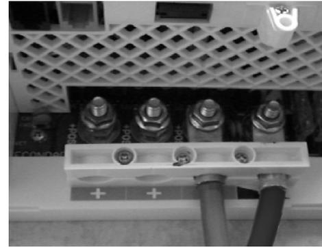
**Please note DC organizer is color coded ensuring proper polarity connections are made.**
