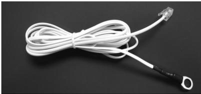
The ProNauticP comes standard with a temperature probe that is plug and play. The temperature probe must be connected while the charger is powered down or before it is connected to the breaker during installation. For best performance, attach the probe to the negative terminal of the "house" batter/bank
