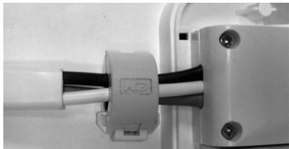
3. Split Ferrite - This split ferrite unit is included with models 1250, 1260 and 2430. It must be installed such that all of the AC cabling passes through it as shown. The split ferrite is to be installed immediately before the AC cable enters the charger.
