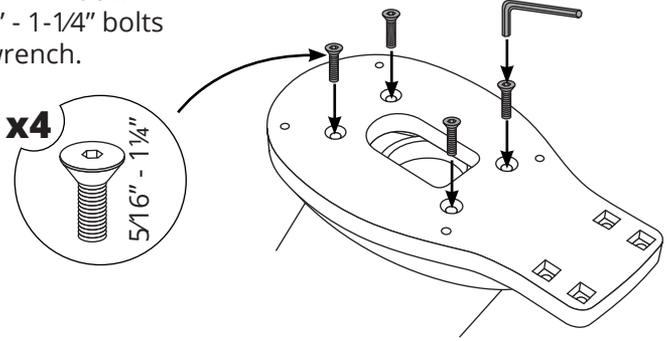
**5** Place the camera on to the ADA-FN-M2 adapter plate.
