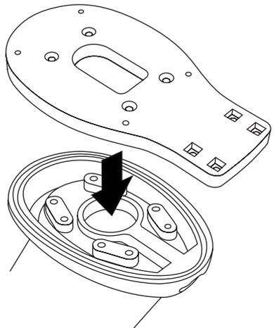
**4** Bolt the ADA-FN-M1 down with four 5/16" - 1-1/4" bolts using an allen wrench.
