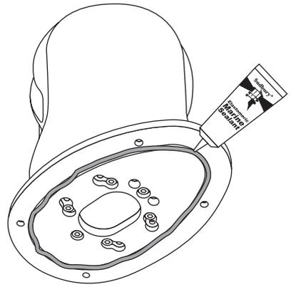
**8** Apply marine adhesive sealant to the four bolt holes. Then bolt the ADA-FN-M2 plate down with four 5/16" - 1-1/4" bolts using a allen wrench.
