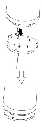
Apply marine adhesive sealant to the ciruclar groove on the underside of the top adapter plate. Route the cables through the adapter plates and rubber grommet. Secure the adapter plates together with the four 1/4-20 x 1" bolts and nylon shoulder washers.
