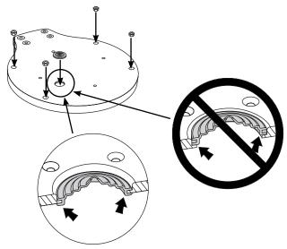
Bolt the dome to the top plate using electronic manufactures hardware recommendation.
