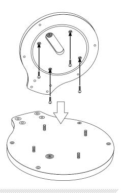
Attach the satellite dome to the adapter plate using electronic manufacturers suggested hardware.
