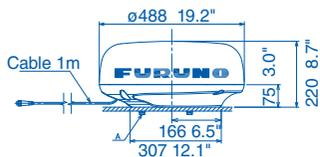
19" Radome Radar Sensor DRS2D-NXT 6.5 kg 14.3 lb
