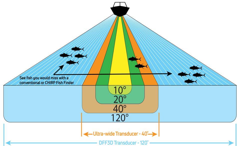
The DFF-3D Multi Beam Sonar operates at 165kHz, giving you fantastic depth penetration while still displaying echoes in high-resolution. Compared to a 40° ultra-wide transducer, you will see 3-times the area around your boat, helping you to find fish you might have otherwise missed. Plus, you can see which side of the boat they are on!
