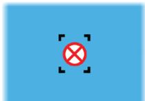
When an AIS SART (Search and Rescue beacon) is activated, it starts transmitting its position and identification data. This data is received by your AIS device.
