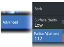
3. Move the position adjustment scroll bar so the top of the **V** in the image is centered at the top of the panel.
