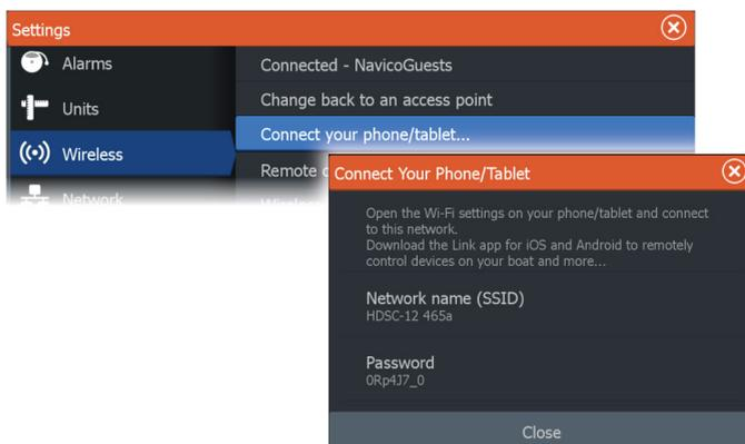
The MFD must be in access point mode to broadcast itself. If not already in access point mode, you will be asked to switch to this mode when you select the connect option in the dialog.
