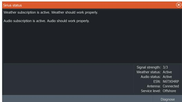
The status panel shows signal strength is indicated as 1/3 (weak), 2/3 (good) or 3/3 (preferred). It also includes antenna status, service level, and the electronic serial number for the weather module.
