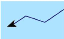
Trails are a graphical presentation of the historical path of the vessel. They allow for retracing where your boat has travelled. Trails can be converted to routes from the edit dialog.
