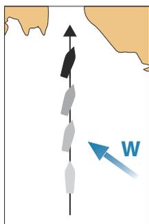
In NAV mode the autopilot automatically steers the vessel to a specific waypoint location, or along a pre-defined route. Position information is used to change the course to steer to keep the vessel on the track line to the destination waypoint.
