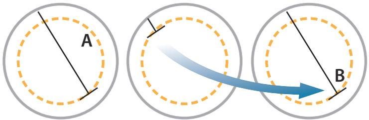
When true motion is selected, the true motion reset option is available from the menu. This allows for manually resetting the radar image and vessel symbol to its starting position.
