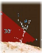
When objects are identified in the water column, they are shown as clusters of dots. The point color corresponds to the target intensity, and the point colors are automatically adjusted to complement the chosen palette.
