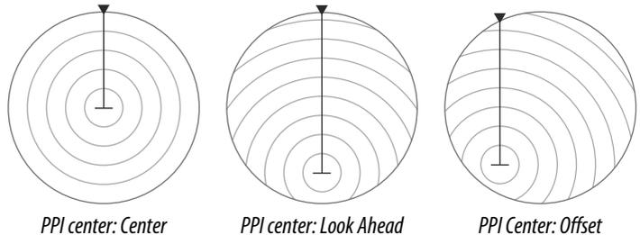
You return the antenna center to PPI center by using the offset option in the View menu.
