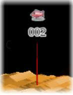
If the cursor is positioned on a 3D image, no depth information is included for the waypoint. The waypoint on a 3D image is drawn with a line beneath it to indicate its point on the sea floor.
