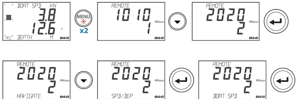
Use the **UP/DOWN** and **ENTER** keys to navigate to a variable and select the variable to display. Exit by pressing the **PAGE** key.
