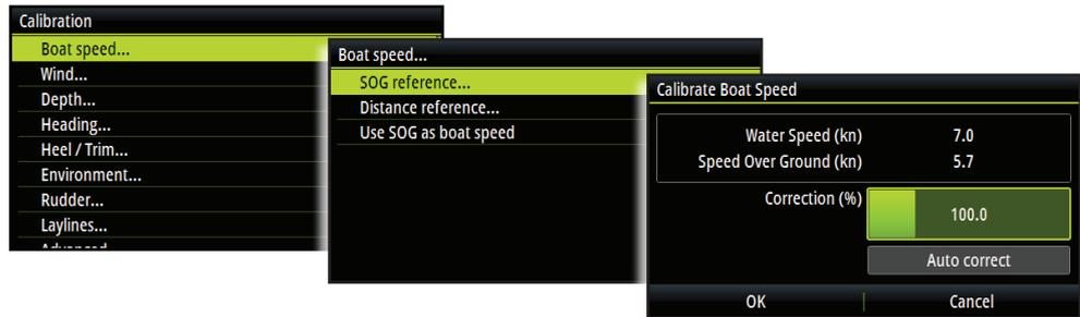
→ **Note:** This calibration should be made in calm sea with no effect from wind or tidal current.
