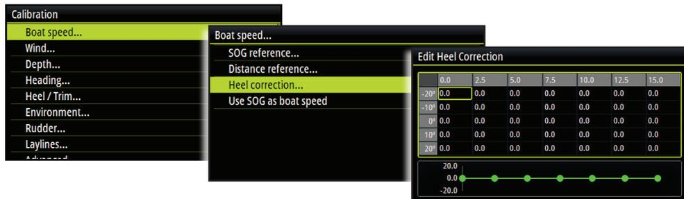
→ **Note:** These options can be set via the H5000 Calibration menu on a compatible B&G Multi Function Display (MFD)
