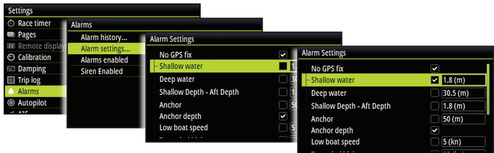
→ **Note:** It is possible to enable / disable all alarms by selecting the 'Alarms Enabled' field from the Alarms menu.
