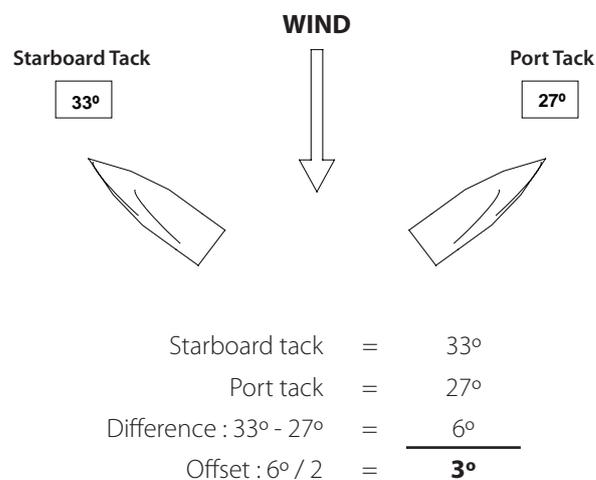
If the starboard apparent wind angle is greater than the port angle then divide the difference by 2 and enter this as a negative offset. If the port angle is greater than the starboard then divide the difference by 2 and enter this as a positive offset.
