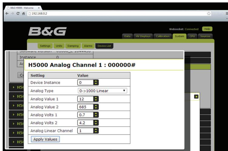
→ **Note:** The recommend calibration procedure for a positional sensor (i.e. Boom Angle, Rudder Angle, Keel Angle etc.) is to move the sensor to its maximum Starboard position, pressing the
