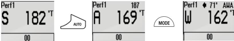
To access other autopilot modes, press and hold the **MODE** key for 2 seconds. Then highlight the required mode and press the **1° >** key to confirm.
