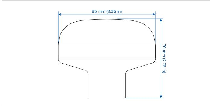
**Important:** If you are replacing a GPS antenna supplied with an older AIS receiver or an AIS700 with an early (low) serial number, please be aware that the mounting diameter (cutout) of the GPS receiver has changed, from Ø44 mm to Ø60 mm.
