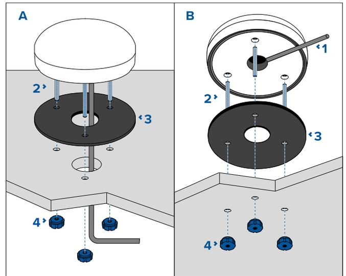
3. Screw the supplied mounting studs (2) into the underside of the antenna.
