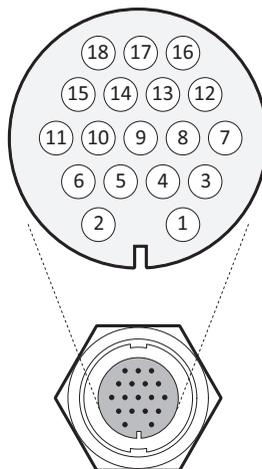
Figure 14 18-Way connector cable wiring connections
