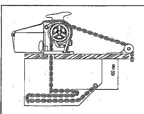
Check there are no deck obstructions. Be sure there is ample room to enable you to use the handle (352). In order to facilitate maintenance operations Lofrans suggest to install the windlass on a removable panel fixed on the deck by bolts.
