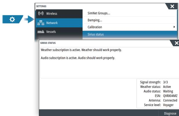
The status panel shows signal strength is indicated as 1/3 (weak), 2/3 (good) or 3/3 (preferred). It also includes antenna status, service level, and the electronic serial number for the weather module.
