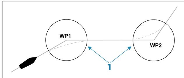
The arrival circle (1) should be adjusted according to boat speed. The higher the speed, the wider the circle.
