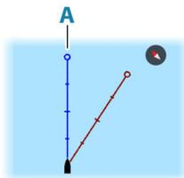
Displays the chart with the vessel's heading (**A**) directed upward. Heading information is received from a compass. If heading is not available, then the COG from the GPS is used.
